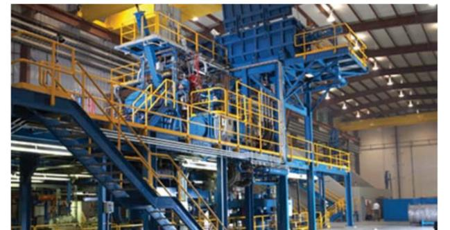
At Perryman, EB melting is used to produce electrodes weighing up to 12,500 lbs.
