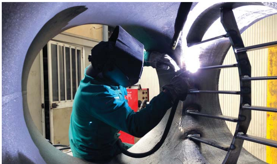
Welding of a barred tee in Petrol Raccord.
