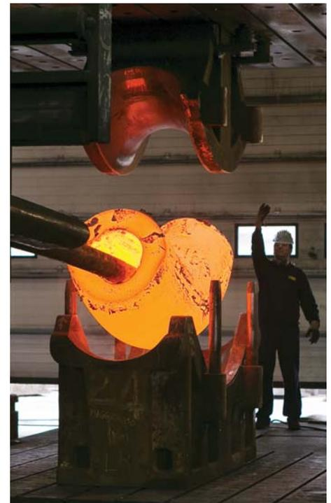
Manufacturing of a large diameter and thickness elbow at Petrol Raccord.
